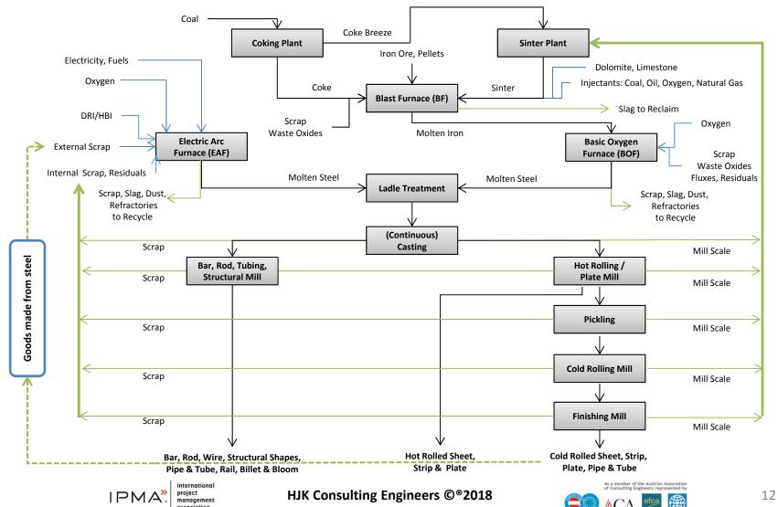
ENERGY SAVING POTENTIALS - Technologies & Measures (samples), Iron & Steel Production life cycle (simplified)
